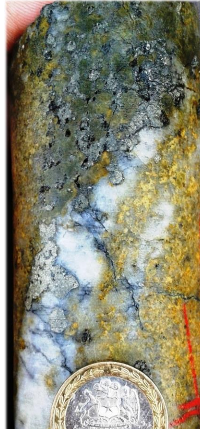
Quartz-Py-Cp±Cc in Crackle breccias in core at Brecha Lipangue Target
